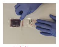
5. Cut open the burst pack at your desired location and squeeze out the ready-to-use adhesive.
