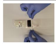
2. Using a hard, son-sharp object, push one component toward the center with light pressure until the separation gives way.
