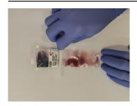
4. Repeat this process until the mass has an even color, or repeat this process at least 20 times for components of the same color.
